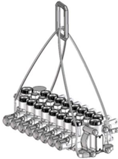
Fig. 5-1 Example of Using Sling
